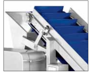
Conveyor belt (above). The outlet (see below) can be regulated and thus ideally adapted to the further process.
